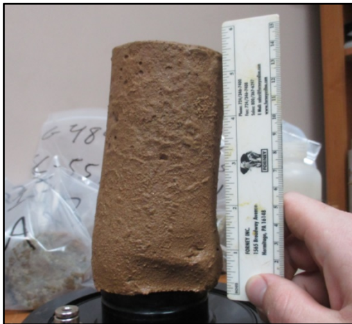
UD-2.A (Sample Slumped on Pedestal)
